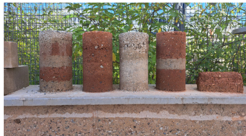
BC Material products: Earth brick masonry and rammed earth commercialised under the "Leem" trademark – examples (Photo: Bas Horsting)
